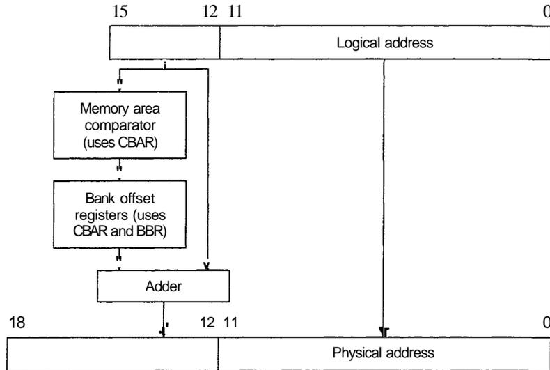
If you use banked memory for the Z80, you must provide decoding circuitry for the ROM banks. The high order address lines (A 12 to A15) must be decoded to select which area of memory is being accessed, and an additional decoder (driven by an I/O port for example) must provide the bank number.
