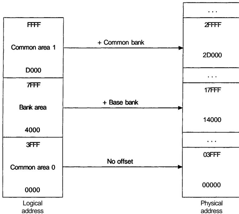
A banked memory model link file (used with linker files 1 nk64b or 1 nkz80b) must be used with a program compiled as banked. The banked function address is based on a three-byte pointer where bytes 0-1 provide the offset and byte 2 is the bank number to supply to the mapping circuit.
