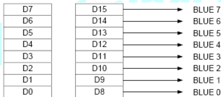
Figure 9: The eight-bit data is wired to BLUE
